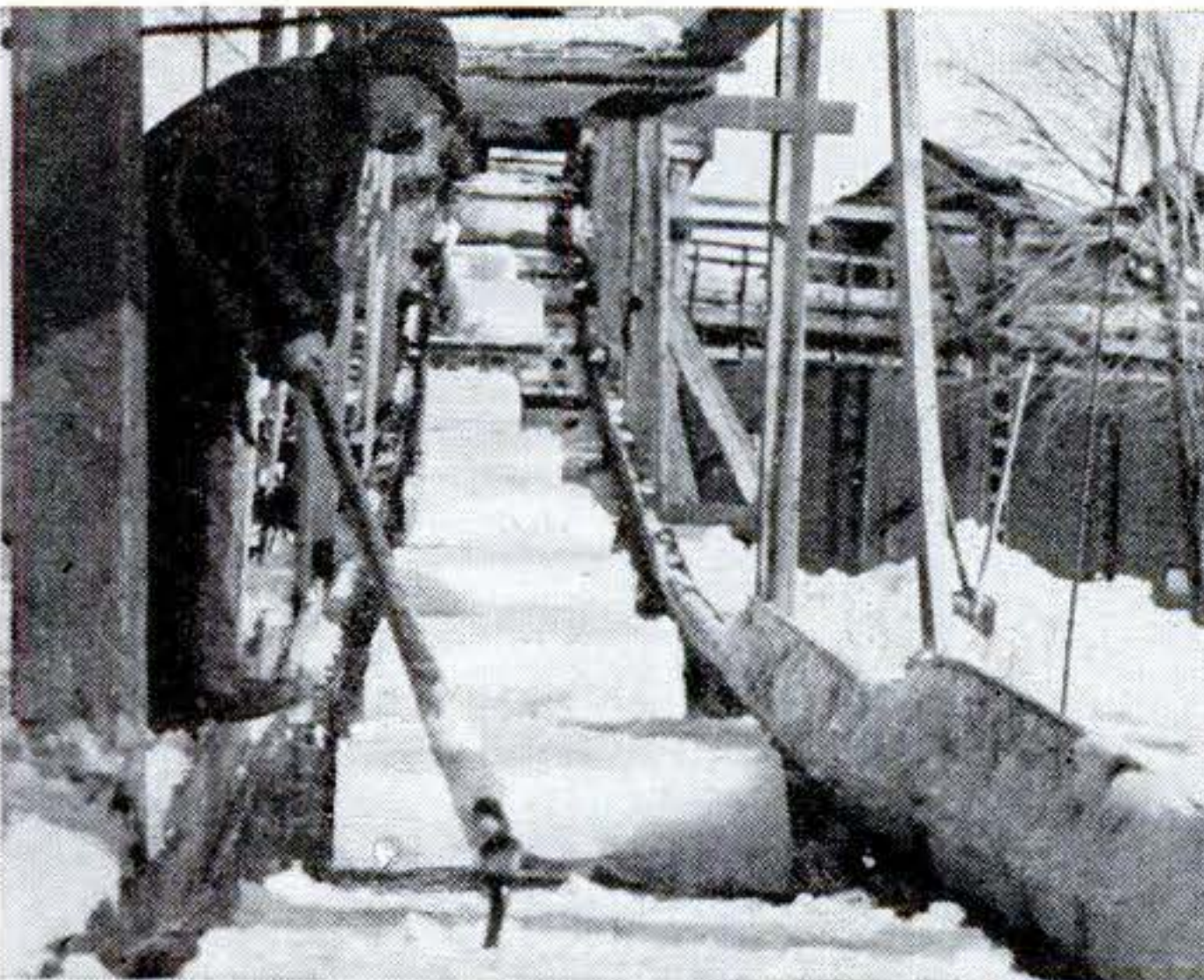
6. Man with pike urges the single cakes onto a conveyer that carries them up to a moving gallery that is adjusted upward as the ice storage house is filled higher and higher.
